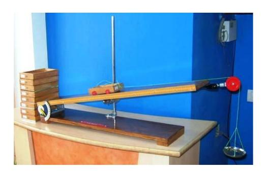
Apparatus consists of a wooden plane 90 x 18 cm having adjustment for setting the angle precisely. Apparatus is supplied complete with a frictionless pulley, linear and circular scale, pan, a wheeled trolley and a set of eight slide draws.
