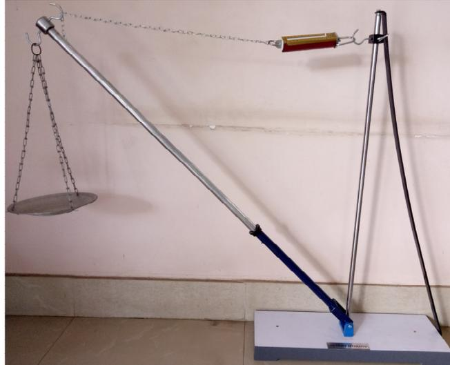
Apparatus consists of a tubular compression balance, pivoted about an axis fitted to the base. The tie chain has an adjustable angle bracket and fitted with a 10 kg extension balance. Apparatus is complete on a wooden base with 1.2m jib.
