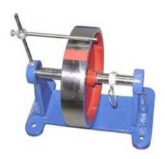
Apparatus consists of a balanced C.I. wheel and the steel spindle is supported on ball bearings in strong iron brackets. The wheel is painted black and is marked with a line. A pointer is fixed to one of the brackets. Diameter hole is drilled in the shaft to take a pin and cord. The base is provided with holes so that the apparatus can be fixed to wall. Apparatus is supplied complete with cord and hook.
