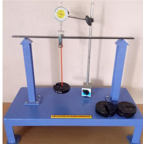
Apparatus consists of a M.S. beam with graduation scale. Supplied complete with two knife edge end supports, a hanger with knife edge and a pointer. Apparatus is supplied with a dial gauge of 25 mm travel with magnetic base and set of weights with hanger.
