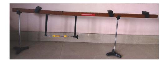
Apparatus consists of a wooden beam 180cm long hinged at a distance of 60cm from one end. A spring balance with adjusting screw compensates the initial extension of the spring and keeps the beam horizontal under any load. Apparatus is supplied complete with three 'U' shaped sliding weights and two knife edge end supports on stands.
